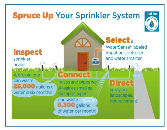
**Inspect.** Check your system for clogged, broken, or missing sprinkler heads. Better yet, go with a pro—find an irrigation professional certified by a WaterSense labeled irrigation program to do the work for you.
